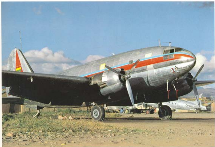
Retractable tailwheel locked and main gears chocked, Super Raton takes a break between operations. Maintenance is carried out in the open as a matter of routine—hangarage is a luxury most Bolivian operators cannot afford or don't need, probably both. Rudderless DC-3 CP-607 in background is owned by Transportes Aereos Tadeo (TAT)
