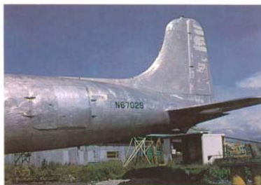
DC-4 N67029 stripped back to bare metal during restoration work at San Jose, California, in September 1983. Overleaf DC-6B N2296B still manages to look majestic despite being parked amid the aeronautical trash at Tucson in February 1984. This airplane is also featured on the front cover
